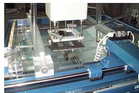
Fig. 3. Experiment setup for measuring dose profiles in water beneath lead skin collimation.
