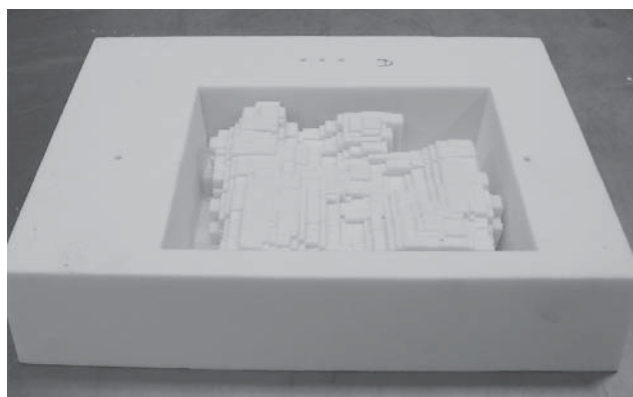
Figure 2. Milled compensator profile. The added holes mark the laser position.
